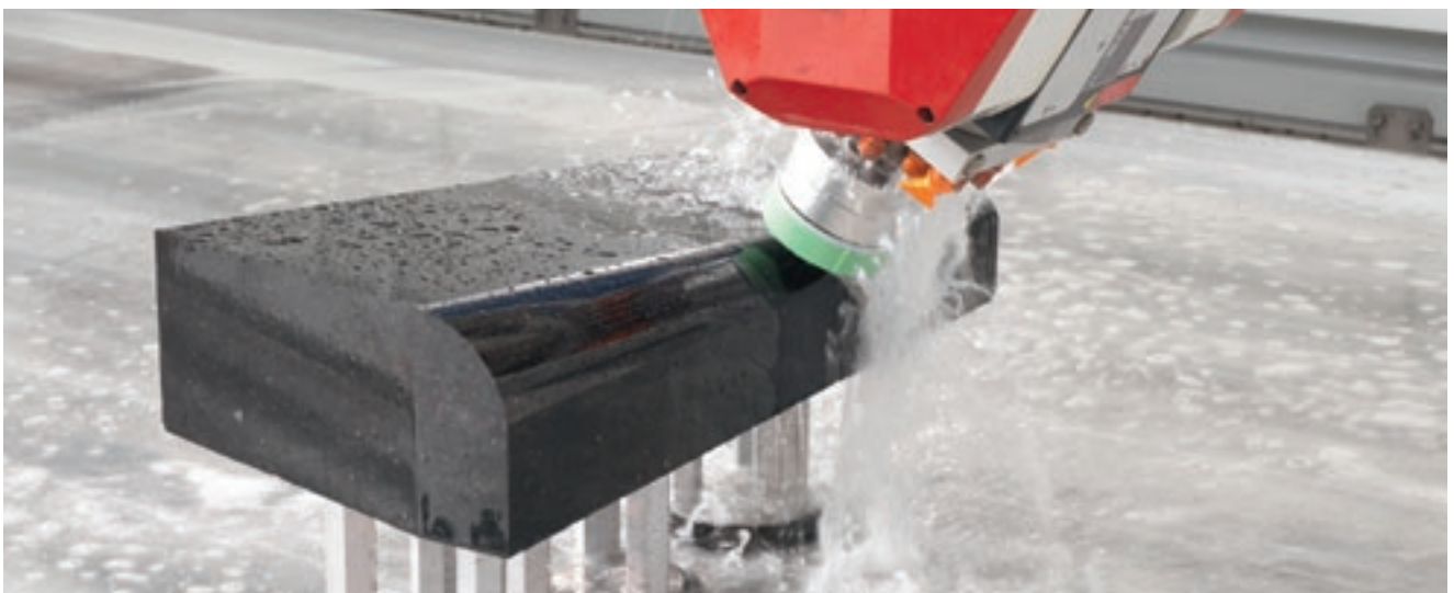
Polishing of rounded profiles on slabs.
