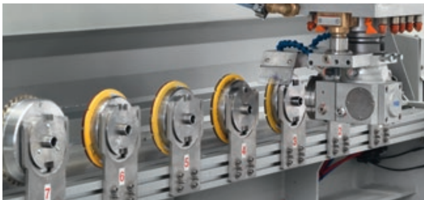
Magazine dedicated to tool change operations for aggregates, with magnetic change.
