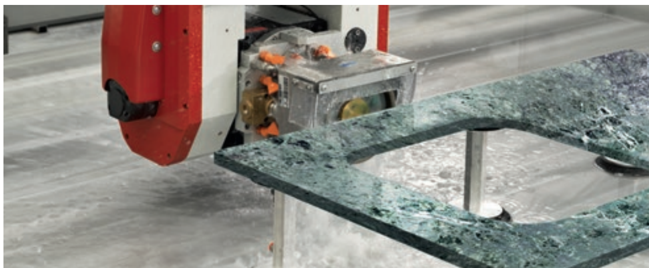
Cup grinding of the external edge.
