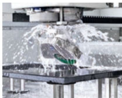
45° disc cuts for joints.
