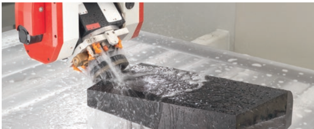
Bevel with variable angle.
