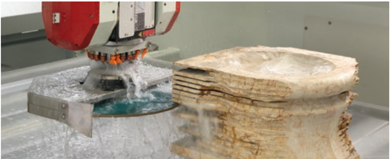
Disc cut at any angle.
